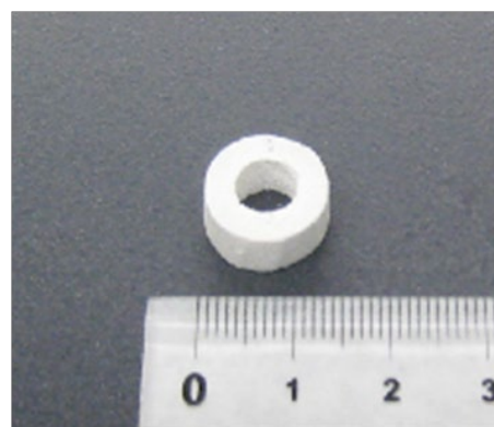
Fig. 2. Photograph of ZSM-5 bulk bodies after trimming and drilling tests.
