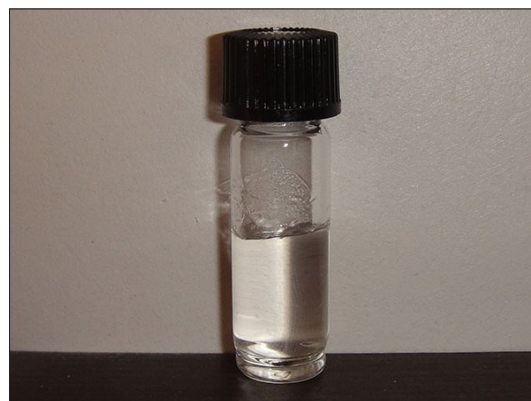
SPG-178 hydrogel. SPG-178 is a synthetic peptide with a neutral pH range. The primary structure is RLDLRLALRLDLR; R = arginine, L = leucine, D = aspartic acid, and A = alanine.
