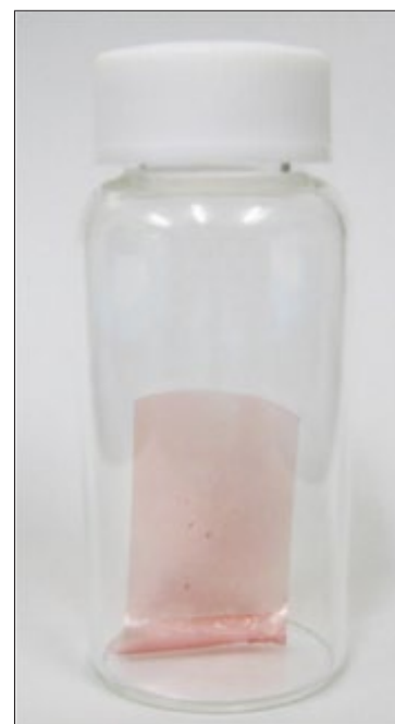
Figure 1. Photoelectric dye-coupled polyethylene film (OUREP™): a novel type of retinal prosthesis.
