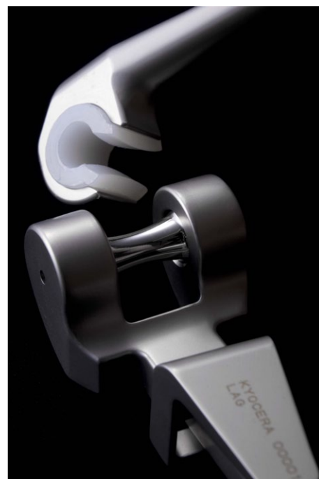
Fig. 2 Articulation of PROSNAP ® elbow prosthesis, showing hand drum-shaped humeral shaft, UHMWPE articulation and sleeve for snap-in fitting of ulnar component.
